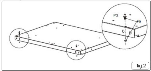
**5.2.** Attach feet to bottom of base as per fig 3
